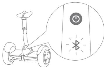
2 Power ON the miniPRO. The Bluetooth icon blinking indicates the miniPRO is waiting for a connection.
