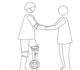
2 Place one foot on the foot mat, with your other foot still on the ground holding your weight. Do not press the steering bar with your leg.
